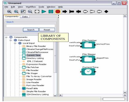
Figure 7: A snapshot of the Kepler environment with the left panel of library components which are loaded at runtime.
