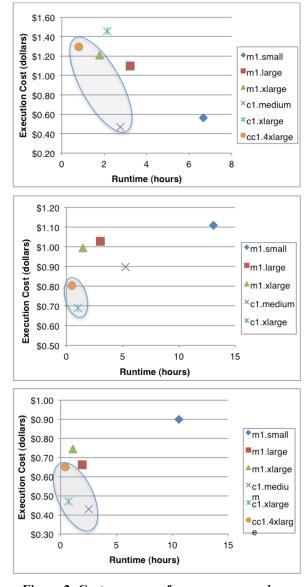
Figure 2: Cost versus performance comparison for Montage (top), Broadband (middle) and Epigenome (bottom). The gray ovals indicate Pareto optimal instance types.
