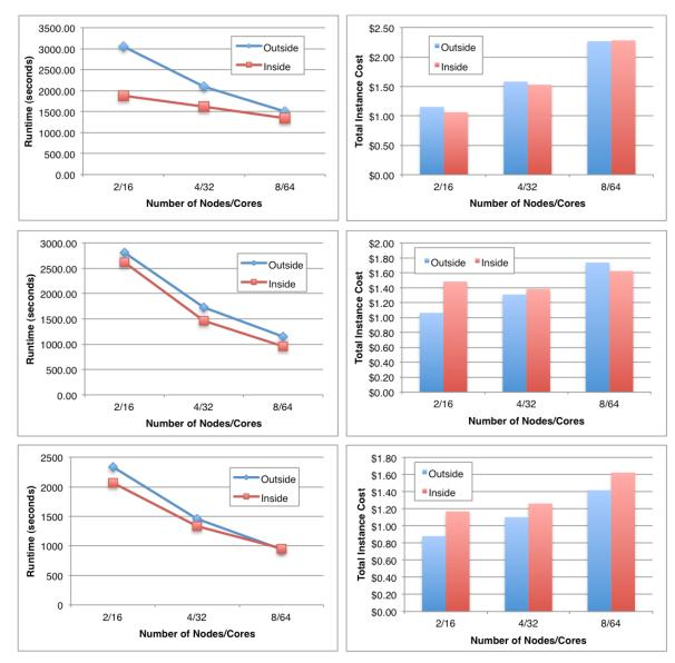
Figure 8: Performance and cost comparison when running the submit host inside the cloud, or outside the cloud for Montage (top), Broadband (middle), and Epigenome (bottom).
