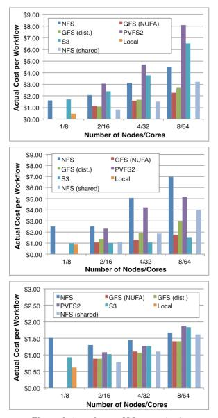
Figure 6: Actual cost of Montage (top), Broadband (middle), and Epigenome (bottom) using different storage systems.
