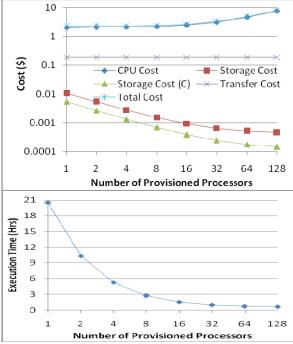
Figure 5. Execution Costs and Execution time of Montage 2
