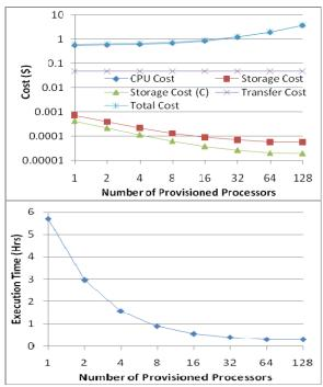
Figure 4. Execution Costs and Execution time for Montage 1
