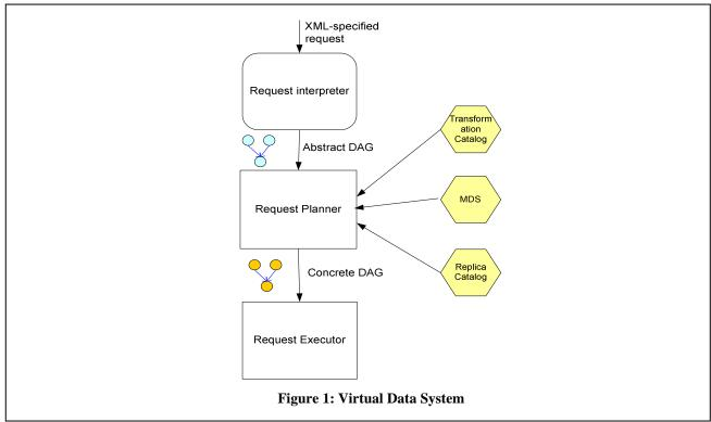
acyclic graph (DAG), is taken by the request planner and transformed into a concrete DAG which includes the commands for necessary data movements, computations, etc. The plan also includes registering new data products in the replica catalog [3] to indicate the availability of the data.
