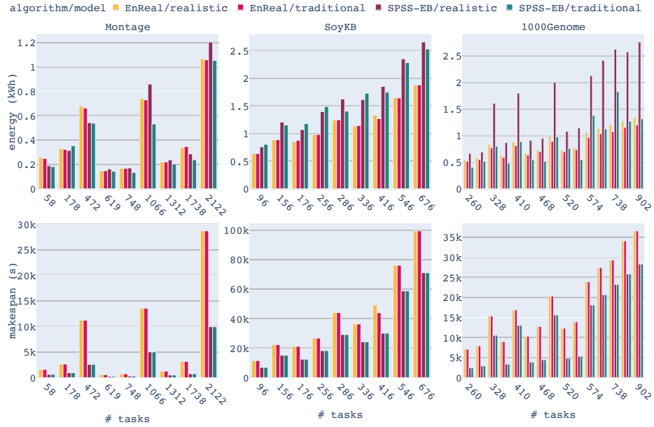
Fig. 1. Simulated workflow energy consumption (top) and makespan (bottom) for each workflow application instance for the SPSS-EB and EnReal algorithms. Results are shown when simulating energy consumption with the traditional power model and the realistic power model.
