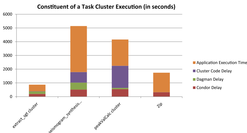
Fig. 15. Average system delays in the execution of clusters and the average application execution time within the clusters. (For interpretation of the colors in this figure, the reader is referred to the web version of this article.)
